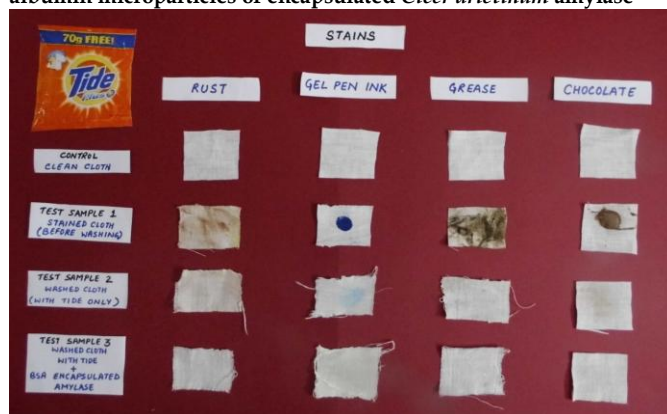
Fig. 6: Washing results of stained cloths with Tide only and Tide with coconut oil driven chemically modified bovine serum albumin microparticles of encapsulated Cicer arietinum amylase
