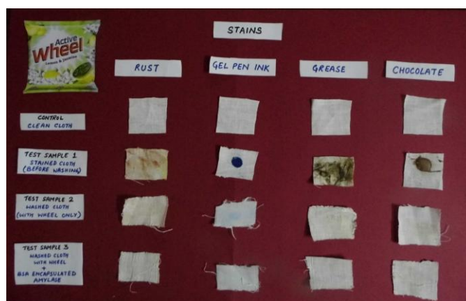
Fig. 5: Washing results of stained cloths with Wheel only and Wheel with coconut oil driven chemically modified bovine serum albumin microparticles of encapsulated Cicer arietinum amylase
