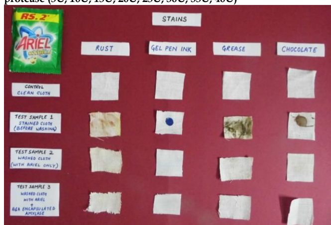
Fig. 3: Washing results of stained cloths with Ariel only and Ariel with coconut oil driven chemically modified bovine serum albumin microparticles of encapsulated Cicer arietinum amylase
